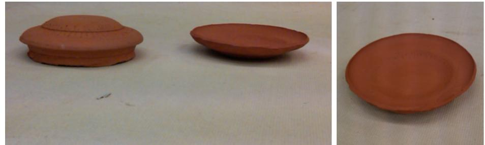
Fired clay hump mould with inscribed decoration and plate off mould
