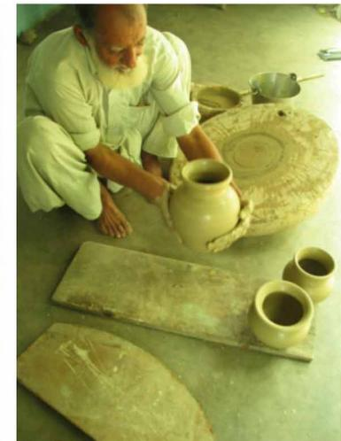
A lump of clay is thrown on the wheel, usually off the hump, making multiple pots from one lump of clay. Simple tools are used; throwing takes a few seconds depending on the shapes. Thrown items include *diyas* (oil lamps), small bowls, and small cups.
