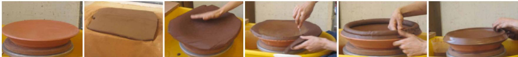
Flat slab press-moulded onto fired clay mould and then trimmed, coil of clay added at the rim and wall pulled
