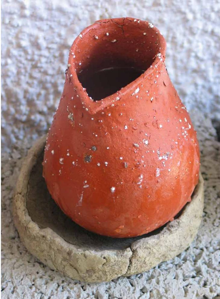
Clay with lime explosions on the surface making it brittle
