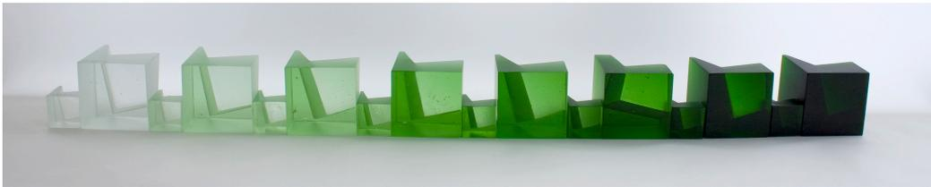
3 cm<sup>3</sup> and 6 cm<sup>3</sup> cubes coloured with chromium oxide. From left: 0.001%, 0.005%, 0.01%, 0.025%, 0.05%, 0.1%, 0.25% and 0.5%.
