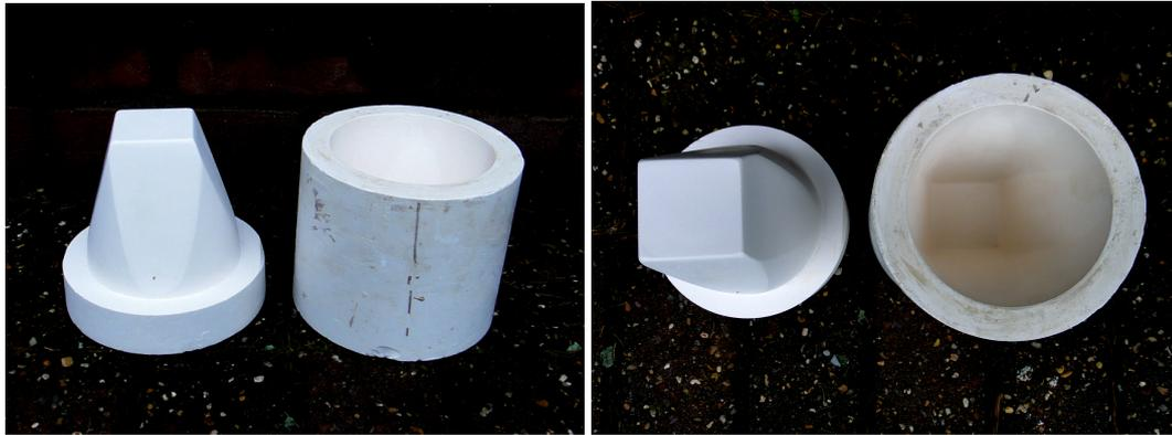
Plug for taking plaster mould off and resulting plaster mould for slip-casting clay kiln casting moulds for basic tests.
