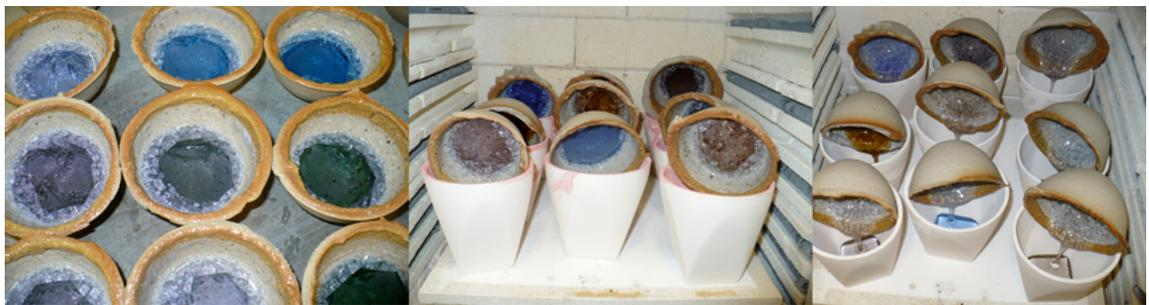
Figure 54: Improved set-up for casting small hue tests.
