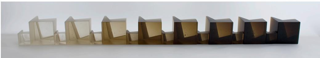
3 cm<sup>3</sup> and 6 cm<sup>3</sup> cubes coloured with nickel oxide. From left: 0.0025%, 0.005%, 0.01%, 0.02%, 0.03%, 0.04%, 0.05%, and 0.1%.
