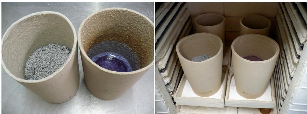
Tall crucible with glass batch, and with glass after firing (left). Crucibles with batch are set up in a kiln on trays with calcined alumina, ready for firing (right).
