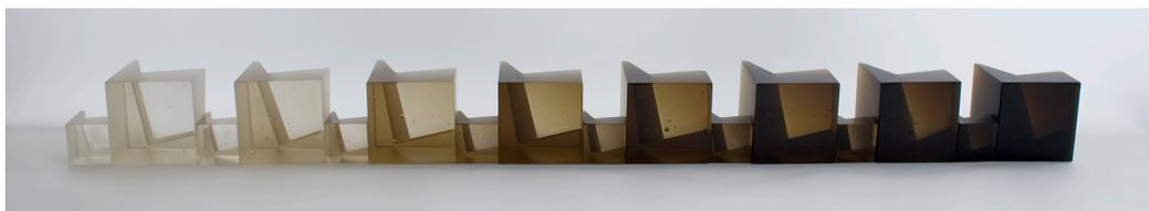
Figure 74: 3 cm<sup>3</sup> and 6 cm<sup>3</sup> cubes coloured with nickel oxide. From left: 0.0025%, 0.005%, 0.01%, 0.02%, 0.03%, 0.04%, 0.05%, and 0.1%.
