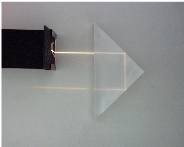
Figure 32: Reflection of light in a Porro Prism
