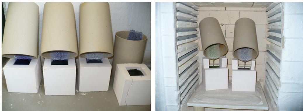
Figure 61: The crucibles adhere to the cast, causing the glass to crack (left). The crucible is suspended above the mould (right).
