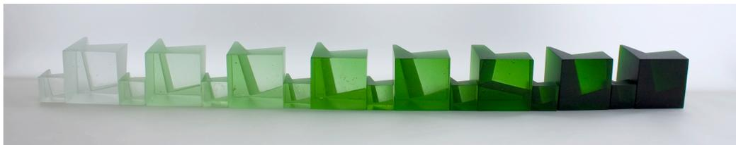
Figure 73: 3 cm<sup>3</sup> and 6 cm<sup>3</sup> cubes coloured with chromium oxide. From left: 0.001%, 0.005%, 0.01%, 0.025%, 0.05%, 0.1%, 0.25% and 0.5%.
