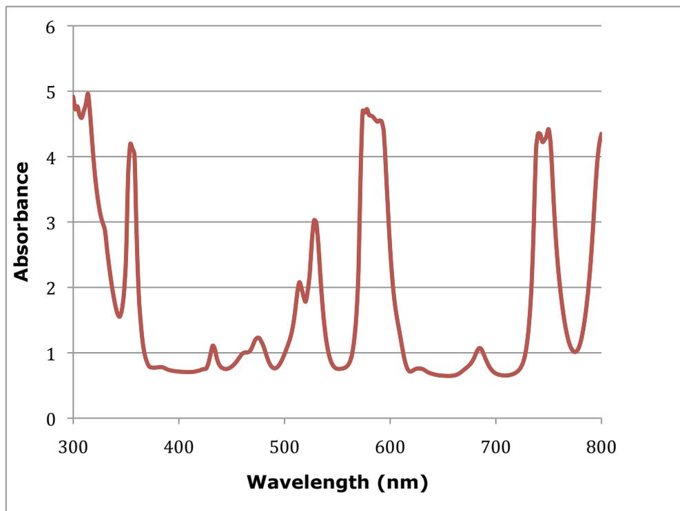
Figure 43: Absorbance of 4% neodymium glass. The graph was generated using a spectrophotometer at Imperial College, with the help of Dr. Ruidong Xia.
