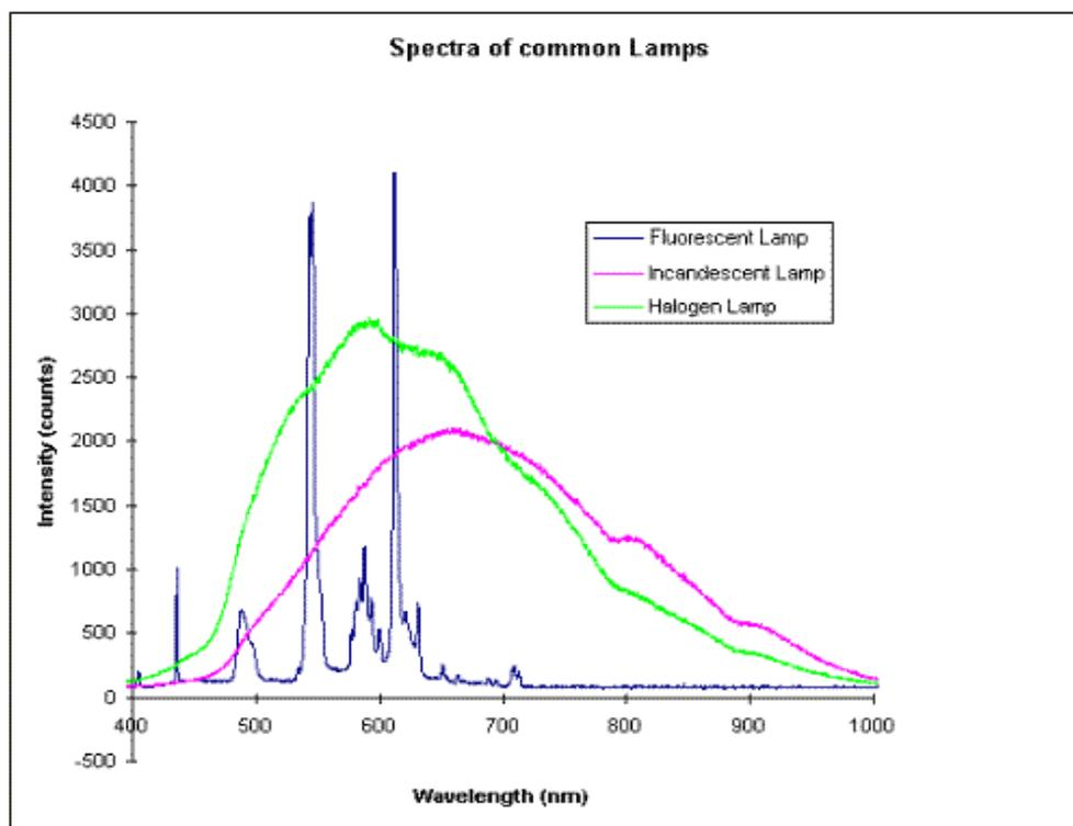
Figure 42: Spectra of common lamps.
