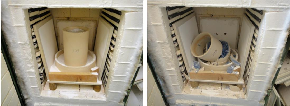
Figure 59: Earthstone handbuilding white ES20 crucible with Glasma frit before (left) and after firing.
