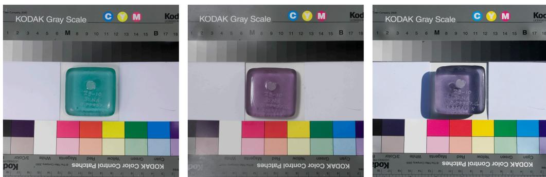
Figure 56: Sample no. 29-10 (3% neodymium oxide, 0.0075% chromium oxide) in fluorescent light, incandescent light and daylight. W: 5 cm.
