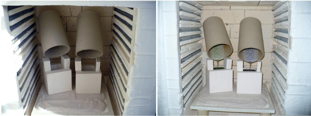
Crucible kiln casting. Before (left) and after the firing (right).
