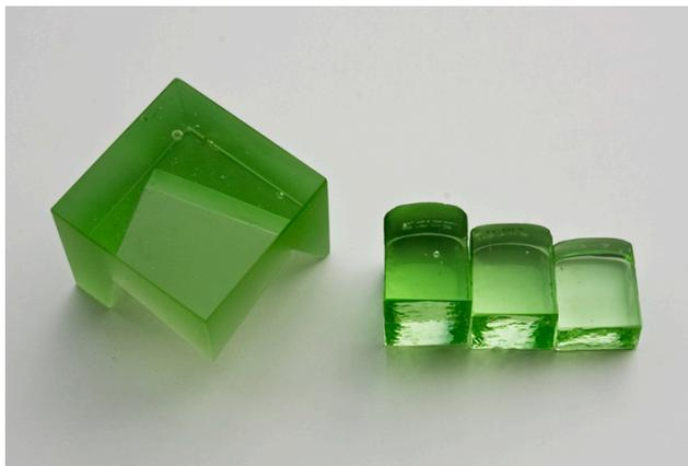
Figure 112: glass coloured with 0.01% chromium oxide. Cube:  $6\text{ cm}^3$ . Thickness of bars: 4 cm, 3 cm and 2 cm.
