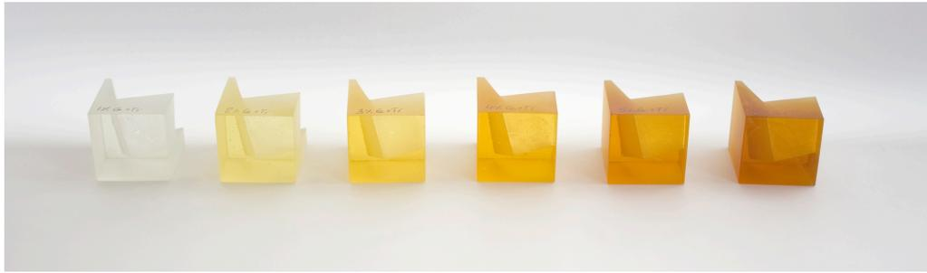
3 cm<sup>3</sup> cubes coloured with cerium oxide and titanium dioxide in the ratio 1:1. From left: 1%, 2%, 3%, 4%, 5%, and 6% of each oxide.
