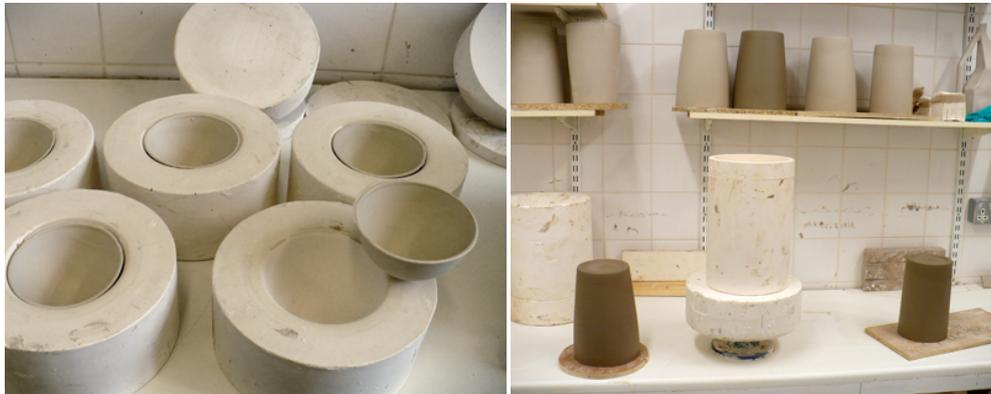
Slip-casting moulds with crucibles.
