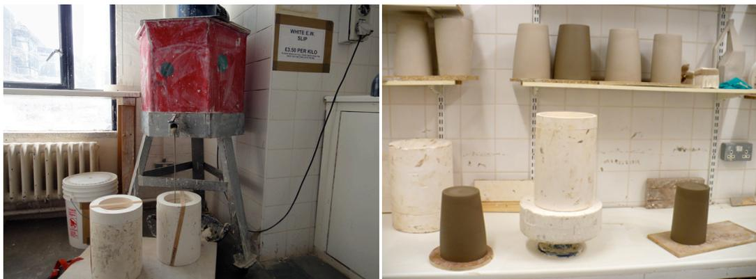
Figure 57: Slip-casting of crucibles.
