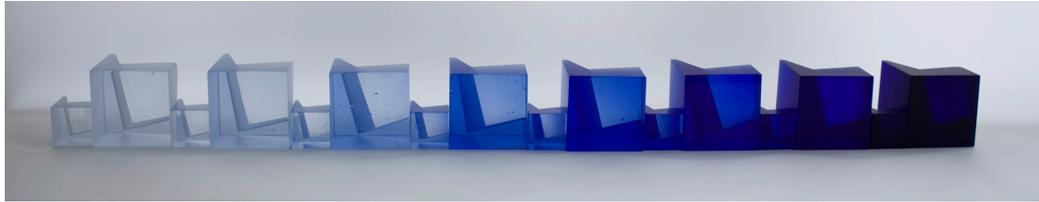
Figure 71: 3 cm<sup>3</sup> and 6 cm<sup>3</sup> cubes coloured with cobalt oxide. From left: 0.00025%, 0.0005%, 0.001%, 0.0025%, 0.005%, 0.01%, 0.025%, and 0.1%.
