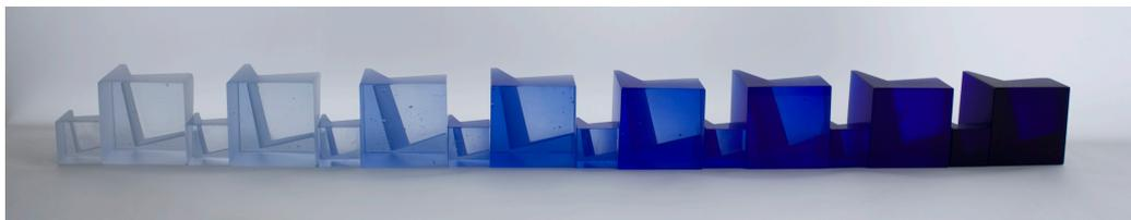
3 cm<sup>3</sup> and 6 cm<sup>3</sup> cubes coloured with cobalt oxide. From left: 0.00025%, 0.0005%, 0.001%, 0.0025%, 0.005%, 0.01%, 0.025%, and 0.1%.
