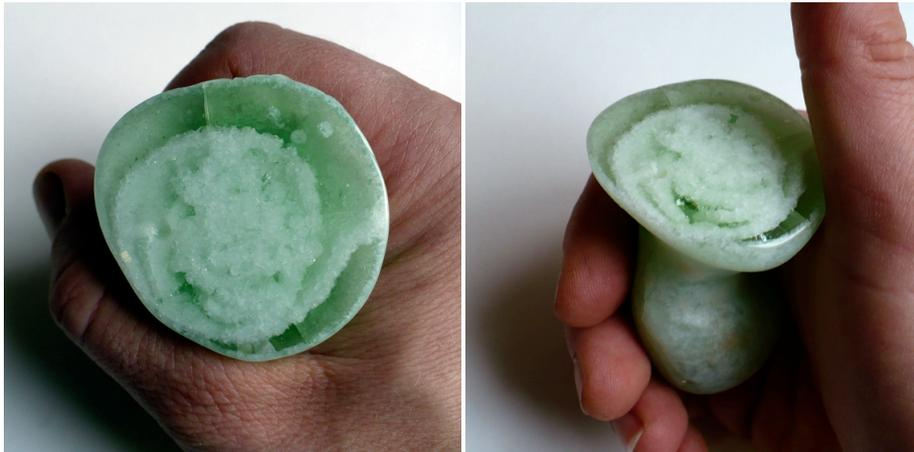
Figure 45: Devitrification in RG2 Glass coloured with 0.01% chromium oxide. Diameter: 4.5 cm, L: 6.5 cm.
