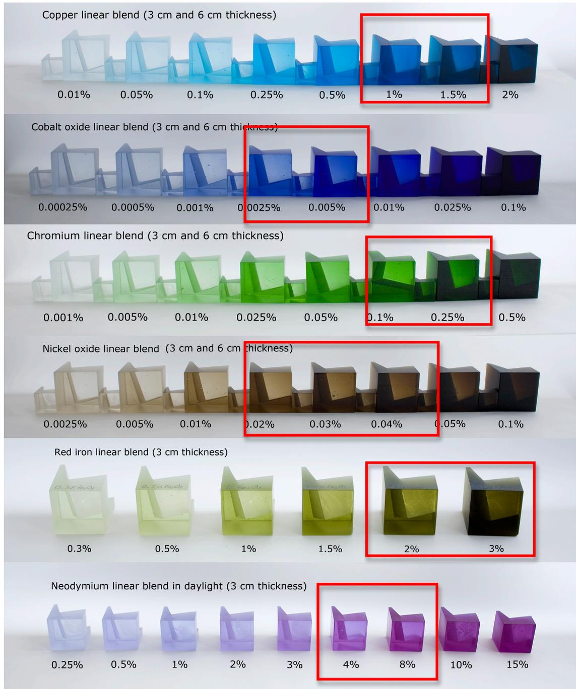
Figure 78: Density thresholds for glass of 6 cm and 3 cm thickness. Cobalt oxide: 0.005%-0.01%; copper oxide: 0.5%-1%; chromium oxide: 0.05%-0.1%; nickel oxide: 0.02%-0.04%; red iron oxide (3 cm): 2%-3% and neodymium oxide (3 cm): 4%-8%.
