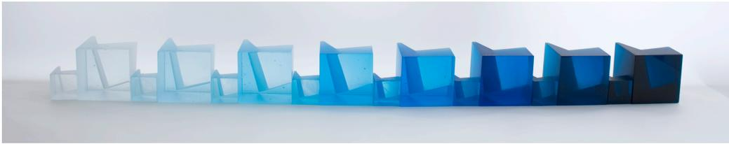
3 cm<sup>3</sup> and 6 cm<sup>3</sup> cubes coloured with copper oxide. From left: 0.01%, 0.05%, 0.1%, 0.25%, 0.5%, 1%, 1.5%, and 2%.
