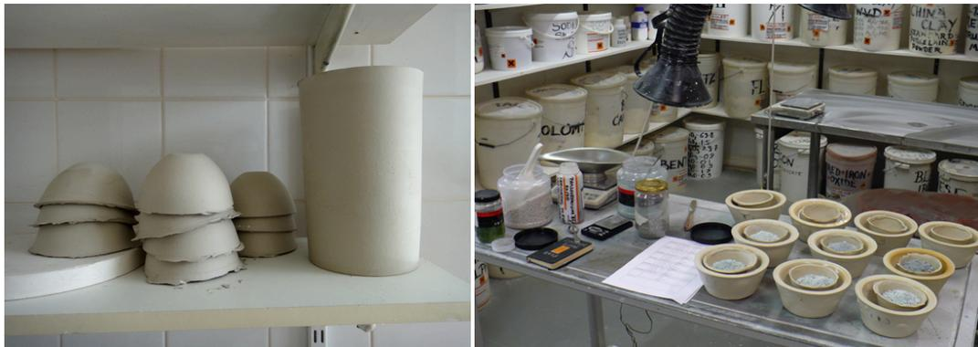
Slip cast and bisque fired crucibles (left). Mixing batch with oxides. The crucibles are placed in trays for firing (right).
