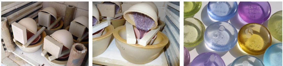
Figure 53: initial set-up for casting small hue tests. Diameter: 5 cm.
