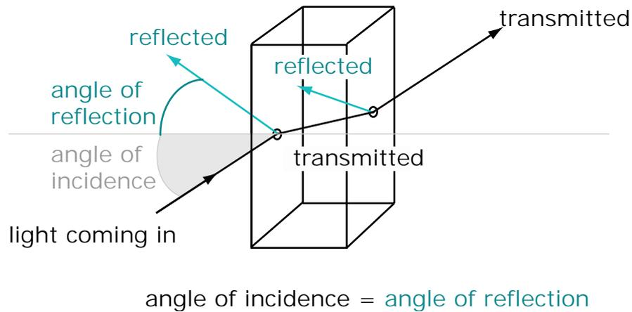
Figure 30: Reflection and refraction
