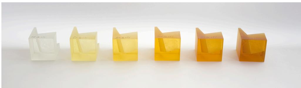
Figure 77: 3 cm<sup>3</sup> cubes coloured with cerium oxide and titanium dioxide in the ratio 1:1. From left: 1%, 2%, 3%, 4%, 5%, and 6% of each oxide.
