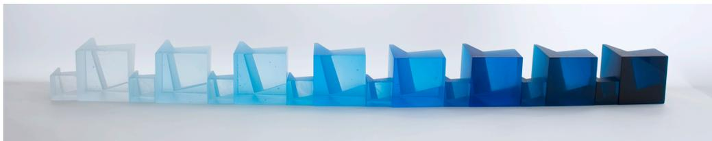
Figure 72: 3 cm<sup>3</sup> and 6 cm<sup>3</sup> cubes coloured with copper oxide. From left: 0.01%, 0.05%, 0.1%, 0.25%, 0.5%, 1%, 1.5%, and 2%.
