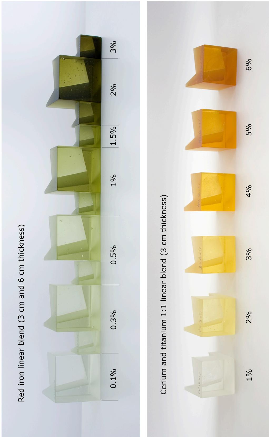
Plate 21: Red iron oxide linear blend; cerium and titanium oxide linear blend, ratio 1:1.
