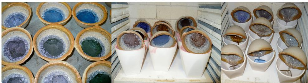
The crucible kiln casting process for small tests.
