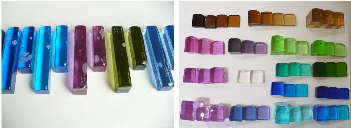
Figure 64: Test bars hot-cast into graphite moulds (left) and cut and polished for spectrophotometer measurements (right). W: 2.5 cm.
